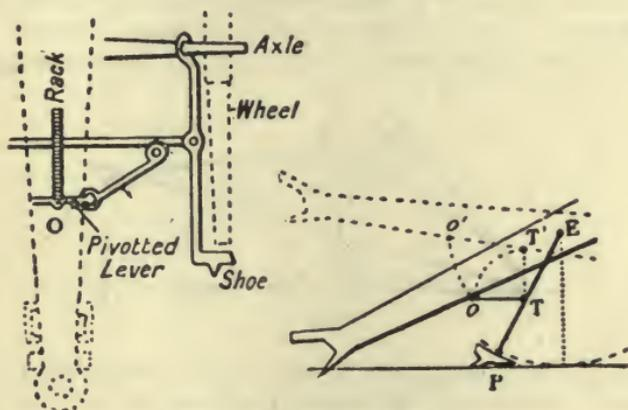
FIG. 3.—Wheel-brake gear.
