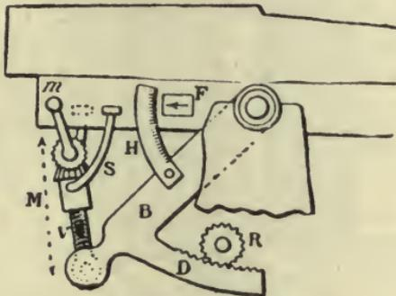
FIG. 5.—Elevating gear.
