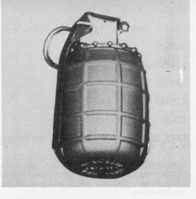
CONSTRUCTION: Plastic body enclosing about 5800 steel balls is fit over an inner plastic cylinder containing the explosive filler,
