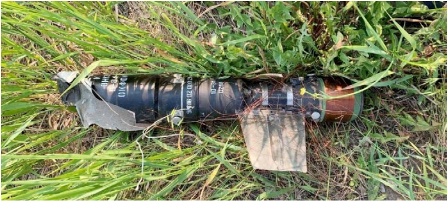
Motor section of fired 9M116. Image © SESU
