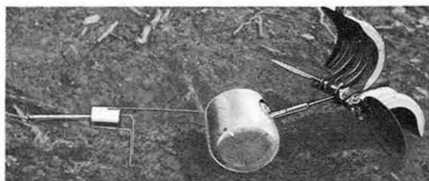
(a) Cavity Charge Mk 2 Mod 0 directed from standoff of four inches for attack on butterfly bomb. High order detonation of the fuze butterfly bomb was obtained.
