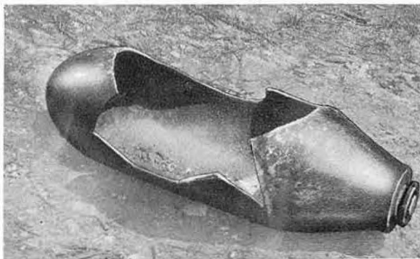
(b) Bomb opened by low order detonation of explosive filling initiated by attack of Cavity Charge Mk 2 Mod 0. The section torn from the case was blown approximately 200 yards.
