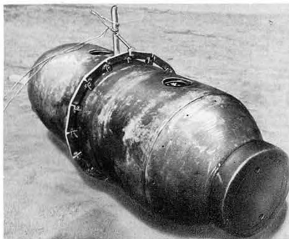
(a) The charges are linked together by means of cotter pin joints incorporated in the standoff legs placed for sectioning of the bomb.
