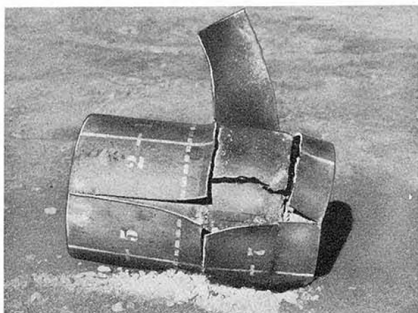
(a) The case of the depth bomb has been split along the weld. The cut section has been peeled back making the explosive that has been chipped loose easily removed.
