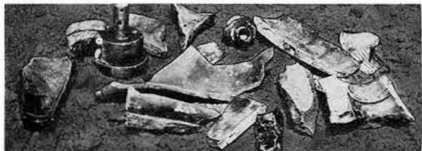
(b) Results of attack on the 8-in./55 A.A. common projectile by the Cavity Charge Mk 2. Sections of the projectile recovered, including the nose and base fuzes, are shown in the picture.
