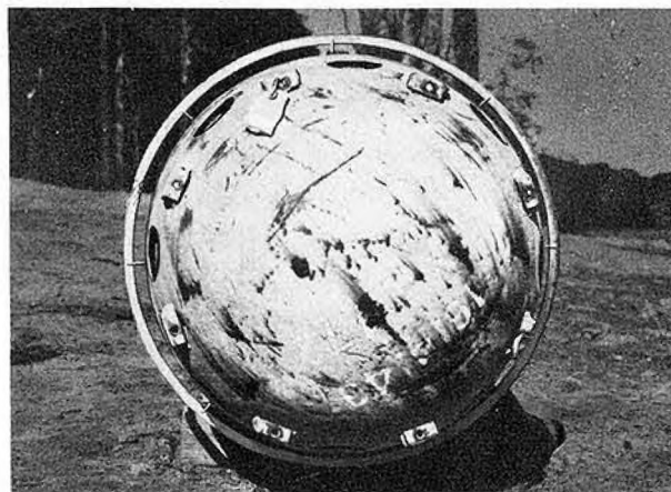
(b) Cavity charge as seen from unit compartment or tail end of the mine. Note the standoff provided by wire legs.
