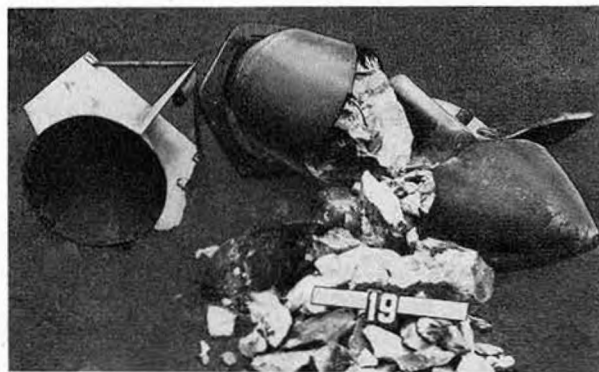
(b) 250-kg. German G.P. bomb opened by low order detonation initiated by attack of Cavity Charge Mk 2 Mod 0. The bomb case is ripped open and the explosive filling is broken up and scattered.
