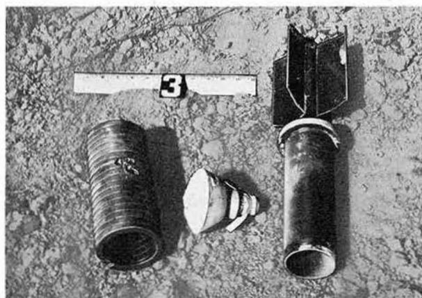
(b) 20-lb. U.S. fragmentation bomb after attack by Cavity Charge Mk 2 Mod 0. Some of the explosive filling still remains in the case which is attached to the tail fins.
