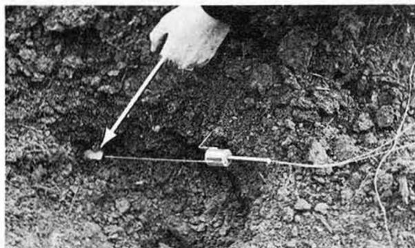
(b) Cavity Charge Mk 2 Mod 0 directed from standoff of eight inches for attack on buried butterfly bomb (indicated by pointer). High order detonation of the fuze butterfly bomb was obtained.
