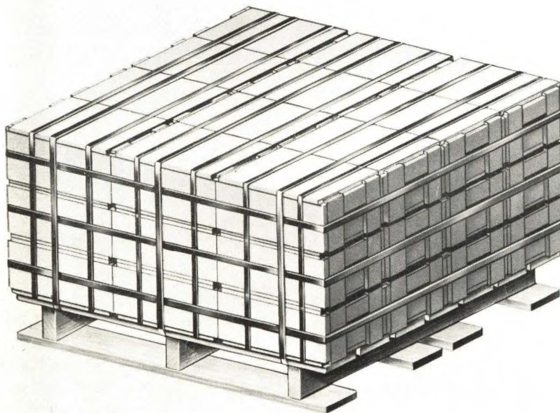
Figure 1-18. Typical Unit Loads of Rocket Components, Showing a Unit of Unpackaged Heads and a Unit of Packaged Heads.
