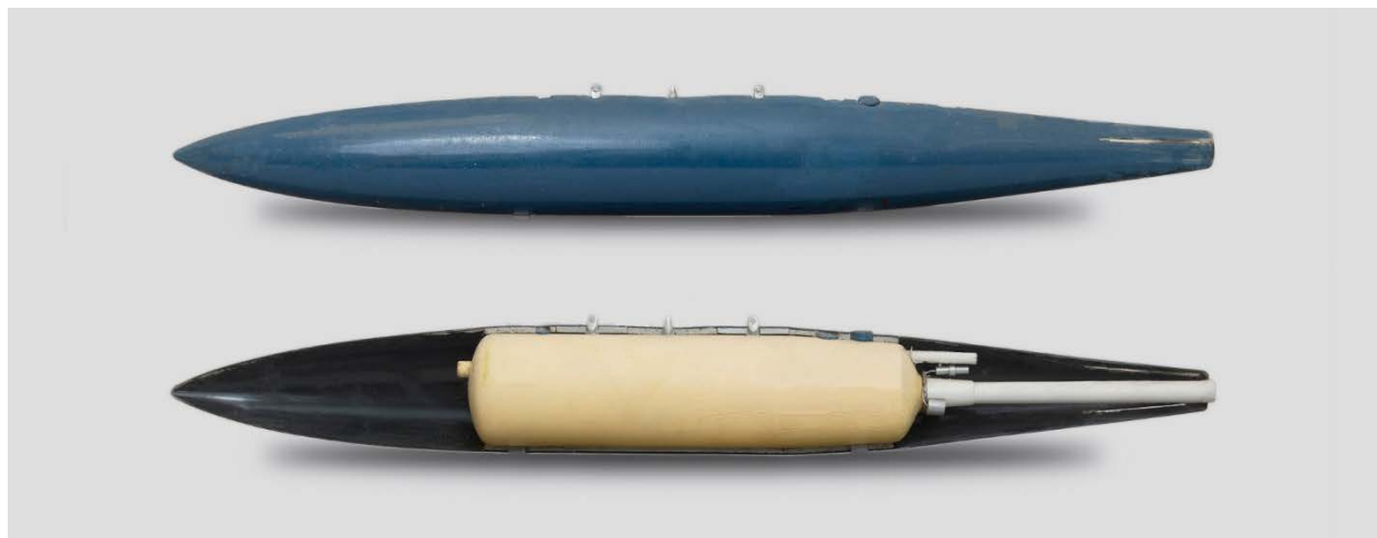
Figure 111: Tank, 84-gallon, Aircraft, Aero 14B - Photograph - Top: Exterior, Bottom: Cutaway View with simulated agent
