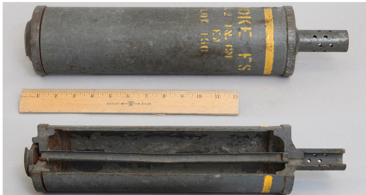
Figure 125: Mortar, 4-inch, MI, Stokes - Photograph - Inert, Top: Cutaway View, Bottom: Exterior
