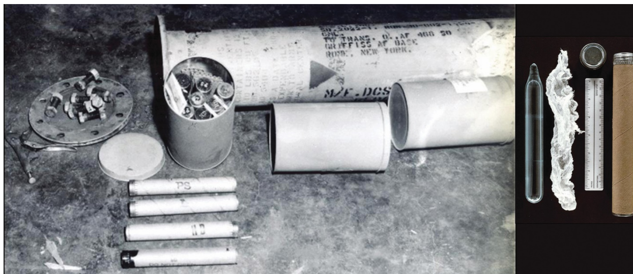
Figure 74: CAIS, War Gas Identification Set, Instructional, K951/K952, M1 - Photograph - K951/K952 Steel Cylinder (PIG) and Contents
