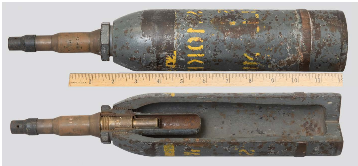
Figure 133: Projectile, 75-mm, MK II - Photograph - Top: Exterior, Bottom: Cutaway View
