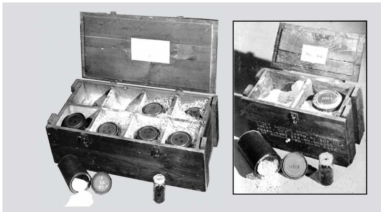
Figure 64: CAIS, Gas Identification Set, Instructional, K955, M1 - Photograph - Left: K955 Components in Box, Right: Navy M1 Replacement
