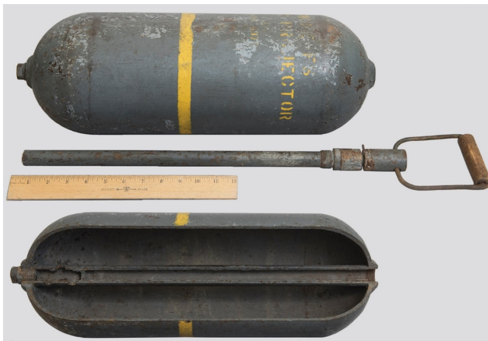
Figure 131: Mortar, 8-inch, Livens Projector, MI, MII, MIIA1 - Photograph - Top: Inert, Bottom: Cutaway
