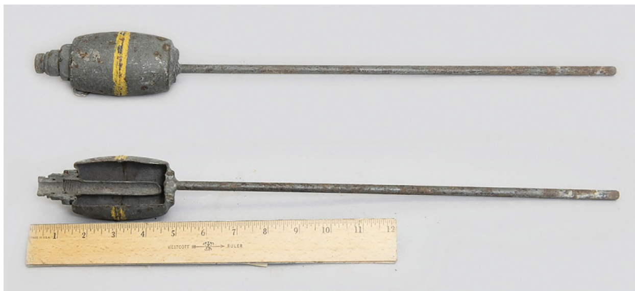
Figure 81: Grenade, Hand, MK1 - Photograph - Rifle projected, Inert without Fuze (note the long rod attached to the base is part of the grenade as designed)
