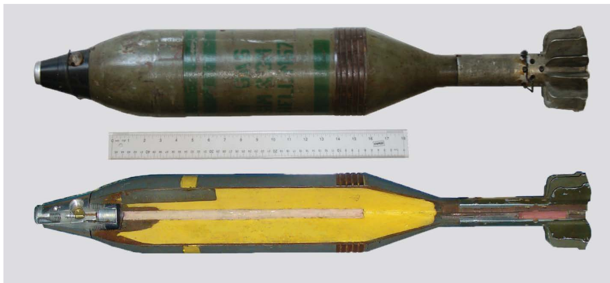
Figure 123: Mortar, 81-mm, M57 - Photograph - Inert, Top: Exterior, Bottom: Cutaway View
