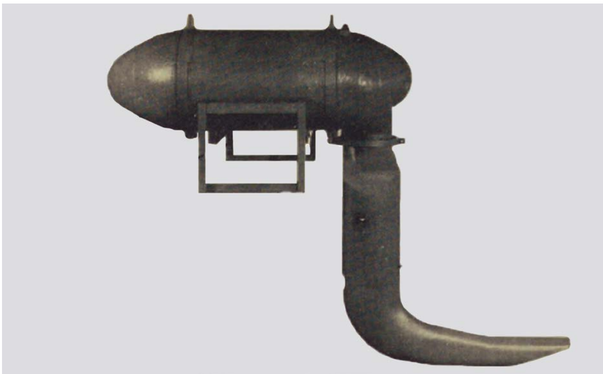
Figure 109: Tank, 70-gallon, Airplane, M33 and AN-M33A1 - Photograph - M33
