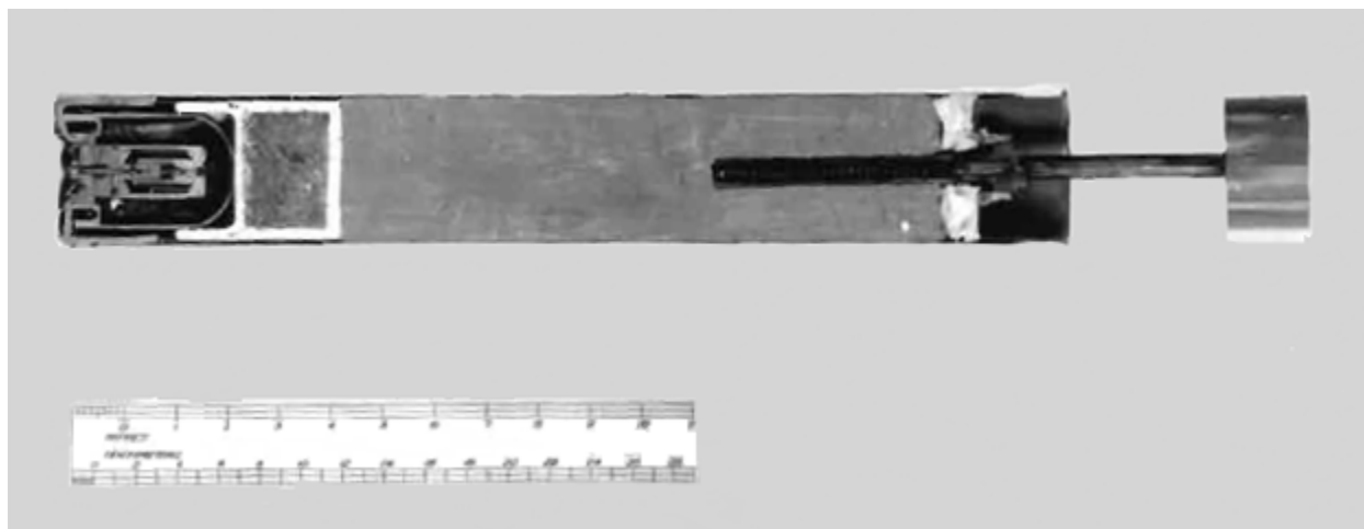
Figure 7: Bomb, 10-pound, M74 (E5), M74A1 - Photograph - Cross Section
