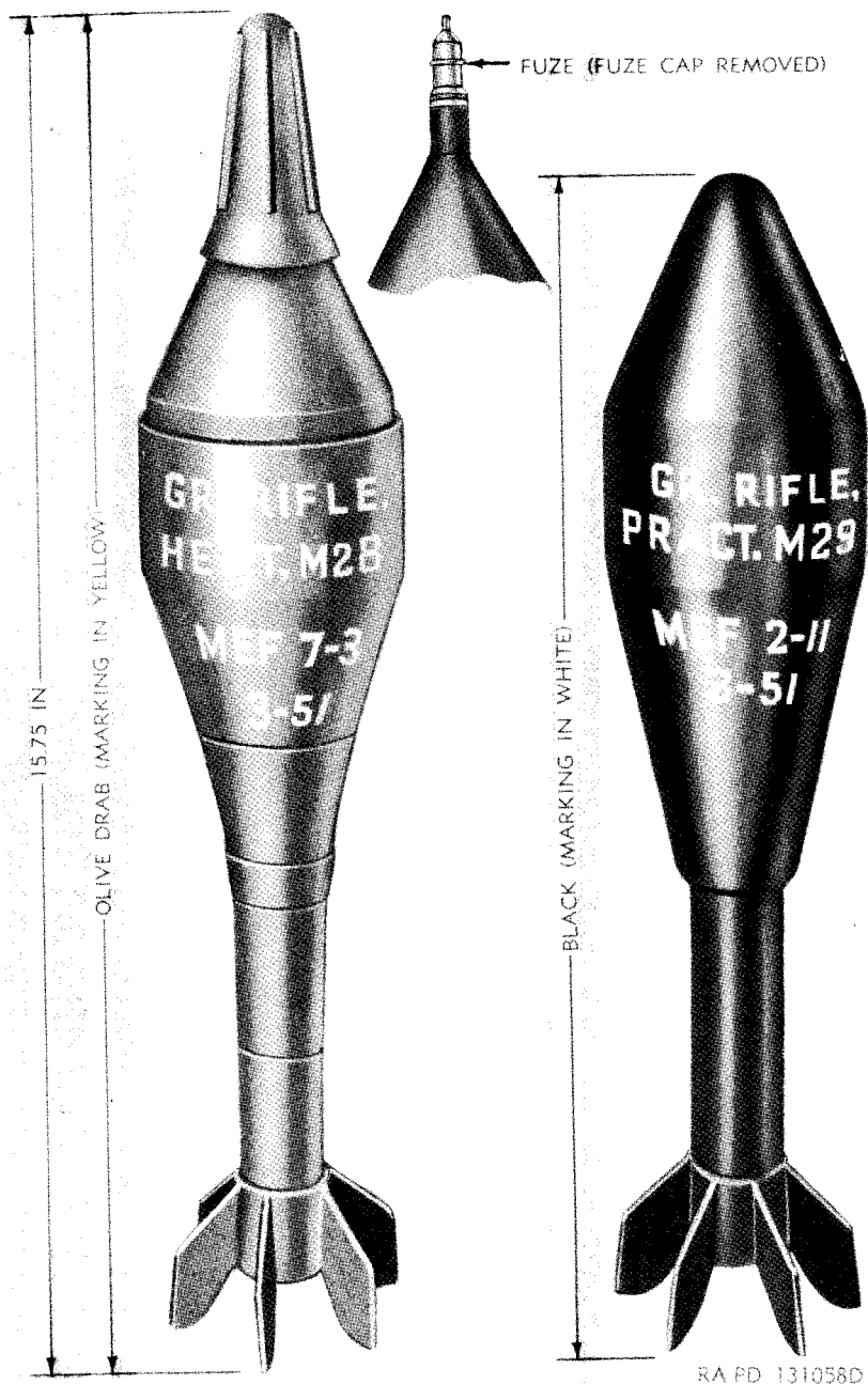
Figure 71. Grenade, rifle, HE, AT, M28 and grenade, rifle, practice, M29.
